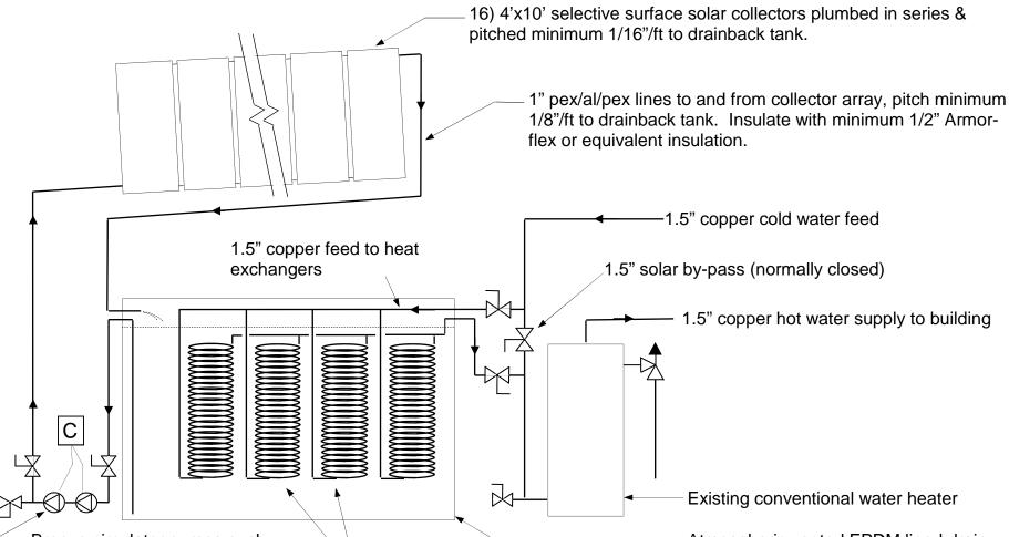
Bronze circulator pumps push water through the collectors. Prewired pumps plug into a pre-wired controller. The controller turns pumps on when the temperature in the solar collectors exceeds the temperature at the bottom of the tank. Stabilized flow through the pumps to be between 8 to 12 gpm.
